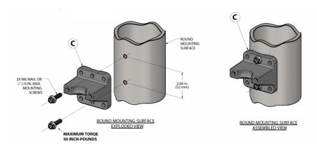
Note the different screw locations for a flat vs. curved surface. The mounting patterns for flat and curved surface are shown below.
